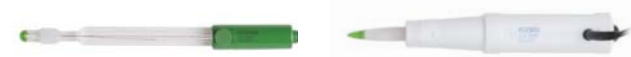
HI10480 PTFE reference, double junction, Clogging Prevention System (CPS), glass body pH electrode with temperature sensor Recommended for wine analysis and solutions with a high concentration of suspended solids FC2320 Open viscolene reference electrolyte, double junction, PVDF body pH electrode with conical tip and temperature sensor Recommended for meat applications with use of optional FC098 20 mm (0.8") or FC099 25 mm (1.4") stainless steel blade
