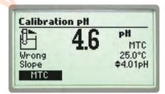
Wrong or Wrong Old Slope – An inconsistency between new and previous (old) calibration is detected.
