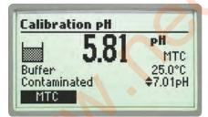
Buffer Contaminated –The offset of the electrode is not in the accepted range. Check if the electrode is broken or clean it following the Cleaning Procedure at the end of this section. Check the quality of the buffer. If necessary, change the buffer.
