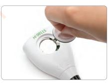
An easily removable cover provides access to the replaceable battery.
