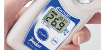
3 Measurement value and prism temperature are displayed in 3 seconds!
