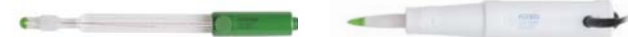
HI10480 PTFE reference, double junction, Clogging Prevention System (CPS), glass body pH electrode with temperature sensor. Recommended for wine analysis and solutions with a high concentration of suspended solids.
