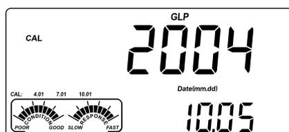
Press the **ARROW** keys to view the next calibration parameter (pressing the **▲** key):
