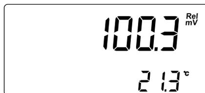
**Note:** Press ← or → from the left keypad to toggle between temperature and absolute mV reading on the secondary LCD.
