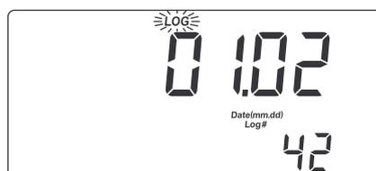
If there are less than 6 memory locations remaining, the record number and "Lo" message will blink for a few seconds to alert the user and then the free locations number is displayed on the LCD.
