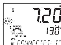
The code and the name of the currently connected probe. If the name was not changed (with Hanna Instruments LAB iPad app) it consists of the last six digits of the SN.
