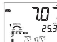
In Standard Mode, Condition gauge is visible on the day of calibration (See Electrode Condition page 29). If configured in SETUP, a countdown message displays the number of days remaining until a new Calibration is due.
