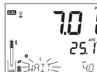
Rinse and submerge the pH electrode approximately 3 cm (1¼") into the second buffer solution and stir gently.
