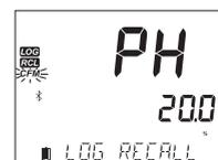
If the percentage is not 0.0%, the user can press **LOG**, and the Export All menu is shown. After the user confirmation, the USB host is activated and the memory stick gets powered. **edge® blu** will start to copy to the USB stick all the available logs.
