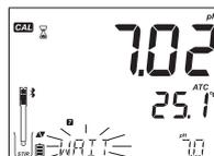
When the reading is stable and close to the selected buffer, "CFM" tag will blink. Press **GLP/CFM** key to confirm calibration.
