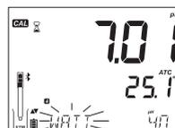
Rinse and submerge the pH electrode approximately 3 cm (1 1/4") into the second buffer solution and stir gently. If necessary, press the  $\blacktriangledown/\blacktriangle$  keys to select a different buffer value.
