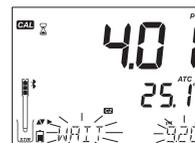
*Note: Custom buffer values can be adjusted  $\pm 1.00$  pH around the set value during calibration. When a custom buffer is displayed, the "C1" or "C2" tag is displayed.*
