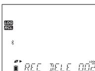
The instrument will display “REC DELETED PRESS CAL TO UNDO”, or RCL to save changes and no measure values will be shown. Multiple records can be deleted. To recover the deleted records, press **CAL/MODIFY** key for each deleted record.
