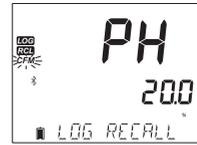
While the pH is displayed and “CFM” blinks and message states “LOG RECALL”, press **SETUP/CLR** key.
