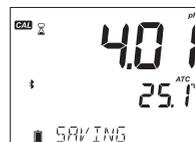
Each time a buffer is confirmed, the new calibration data replaces the old data for the corresponding buffer or for any buffer in the proximity of  $\pm 0.2$  pH.
