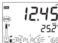
Press the  $\blacktriangledown$   $\blacktriangle$  keys to select another buffer to be replaced.
