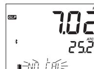
After the calibration has been performed, the instrument displays offset and slope. The GLP slope is the average of the calibration slope; the percentage is referenced to the ideal slope value at 25 °C. Additionally, the condition and response indicators displayed are from the last calibration.
