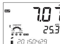
*Note: If a custom buffer was used in calibration, the "C1" and "C2" tags will be displayed. If only the one buffer is used in calibration, the tag will be "C1" and the value will be displayed.*
