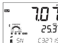
If a buffer is not from the last calibration, the buffer tag will be displayed blinking. If the calibration date and time are not in sync with the current date and time set on meter, the message "Inconsistent GLP time stamp" will be displayed.
