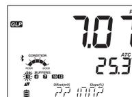
Pressing the  $\nabla$   $\blacktriangle$  keys, the last calibration date (yyyy.mm.dd) together with the current reading is displayed.
