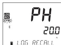
If no data was logged for the selected log type, the instrument displays the following messages (ex. for pH range):
