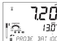
*Note: If GLP/CFM key is pressed the HALO™ LED's on the connected probe will pulse 4-5 groups of fast flashes then return to normal operation. This may be useful to identify the operating probe from a group of probes.*
